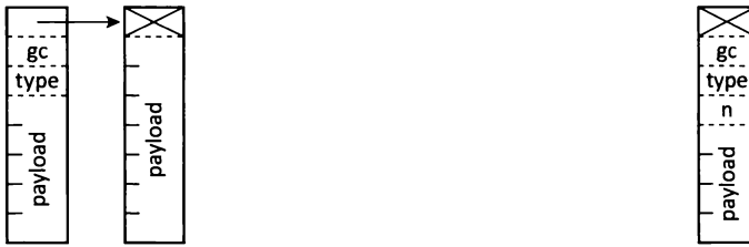
(a) A two-fragment object with a payload of six to twelve words. The sentinel fragment has three header words: a fragmentation pointer to the next object fragment, a garbage collection header and a type header. Each fragment has a header pointing to the next.
